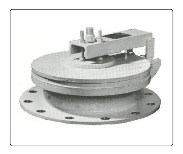
The Emergency Vent (Figure 4210) is an economical solution to the present day emergency venting requirements. It is not intended as protection against an internal explosion, but to prevent excessive vapour pressure rise in the event of an external fire. It is available for use in normal, chemical or low temperature service.
