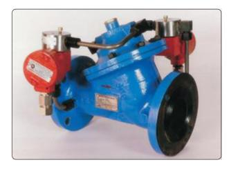
Initially both NO and NC solenoid valves are in deenergised condition. The NO valve applies high upstream pressure on the diaphragm, whereas the NC valve prevents this pressure from getting drained to the downstream side. The valve remains close as a result of this
