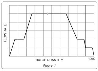
When the flow rate reaches an intermediate stage, NC solenoid valve is de-energised. This stops relieving of pressure in the piston chamber and the valve locks at the current flow rate.
