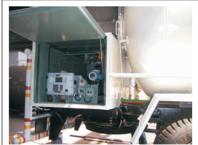
TISI Batch Controller on LPG Truck
