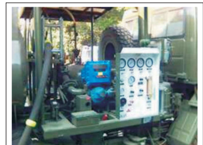
Meter on Aircraft Refueller
