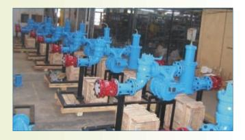
The Skid is cabled, assembled and tested in VERMONT's factory and then delivered to destination.
