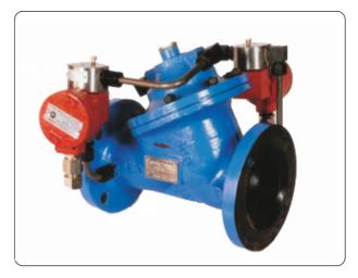
Initially both NO and NC solenoid valves are in deenergized condition. The NO valve applies high upstream pressure on the diaphragm, whereas the NC valve prevents this pressure from getting drained to the downstream side. The valve remains close as a result of this.
